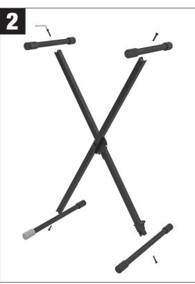
Tighten the arms and legs by the allen key provided and complete set up.
